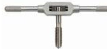
Tap wrench - cuts an internal thread
