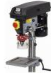
Pillar drill - accurate holes
