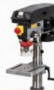
Pillar drill – rivet holes
