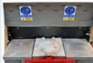
Brazing hearth – heats metal for dip coating
