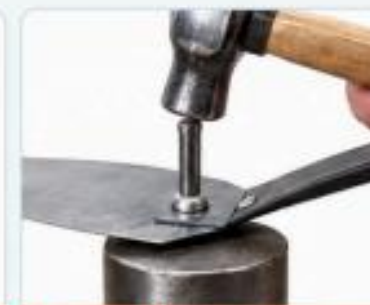
Cold riveting – dome underneath on a dolly
